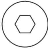
PART# 08 ALLEN HEAD BOLT M12X20L FULL THREAD QTY.2
