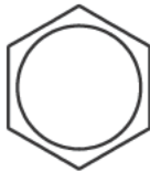
PART # 55 HEX HEAD BOLT M10X65L PARTIAL THREAD QTY.2
