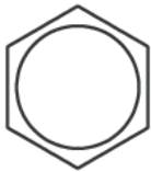
PART # 56 HEX HEAD BOLT M10X90L PARTIAL THREAD QTY.1
