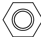
(A5)HEX BOLT M10X60L PARTIAL THREAD QTY.4
